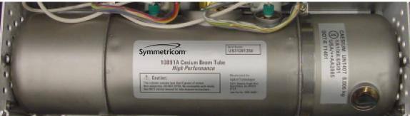
When shipping a 5071A or a replacement CBT in accordance with IATA international DG rules, check the instrument for the above marking. If the marking is present (visible through the cover perforation), follow the IATA international shipping instruction given elsewhere in this website. If the marking is missing, download from this website. Affix it to the CBT as shown. Follow the shipping instruction referenced above.
